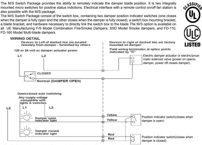
Detailed wiring diagrams including terminal designation and/or wire color coding furnished with each shipment.
